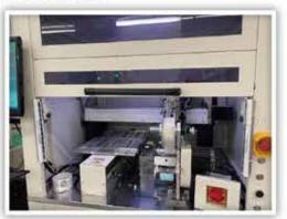
Add photoelectric sensors to the chip mounters to prevent work injuries caused by misoperation
